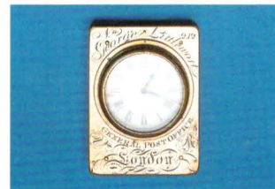
NPM 96/7 Mailcoach guard’s timepiece. The mechanism was wound up, the time set and the timepiece locked at the beginning of the journey. This prevented the guards or postmasters along the route altering the time of the coaches’ arrival and departure and ensured the coaches kept to their strict timetable. Made by George Littlewort.
